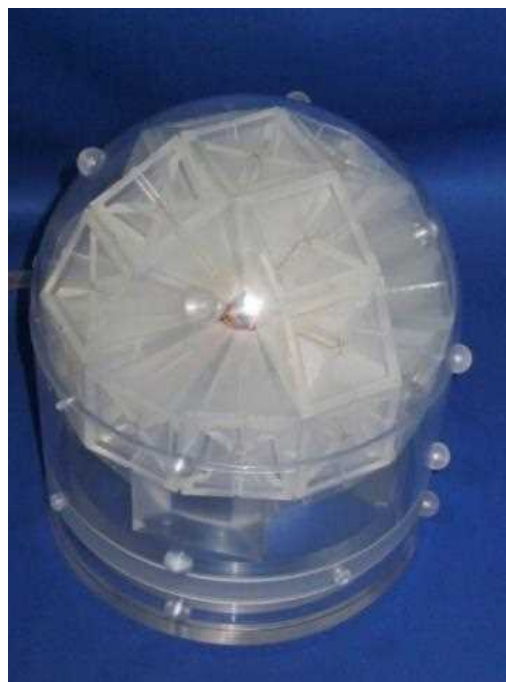
Fig. 4.13 Photograph of the MEG phantom, which has 50 equivalent current dipoles.
