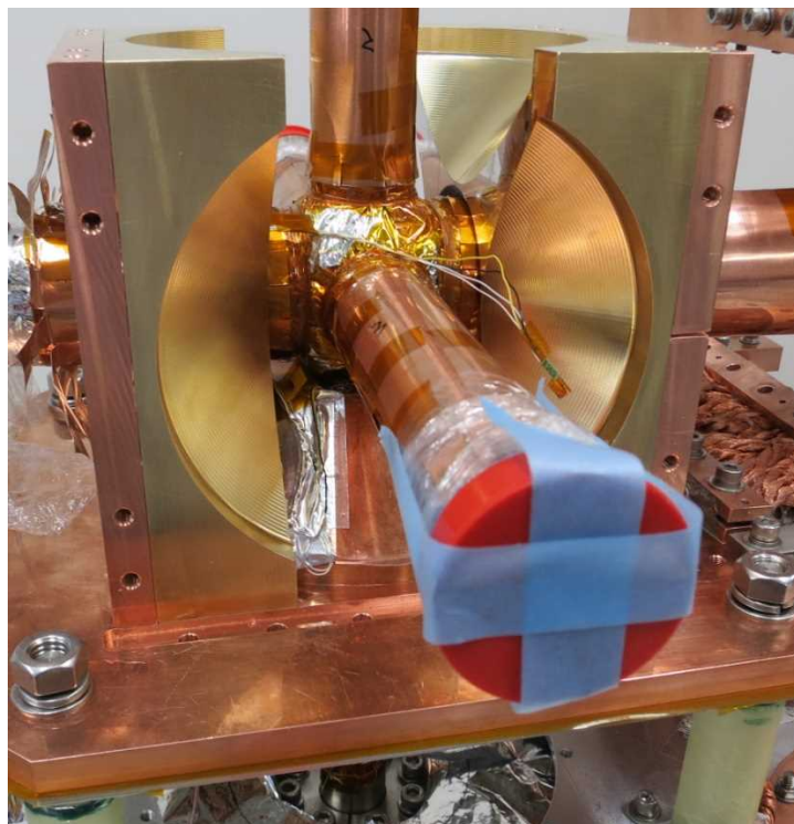
Fig. 3.17 Photograph in installing the brass support block.
