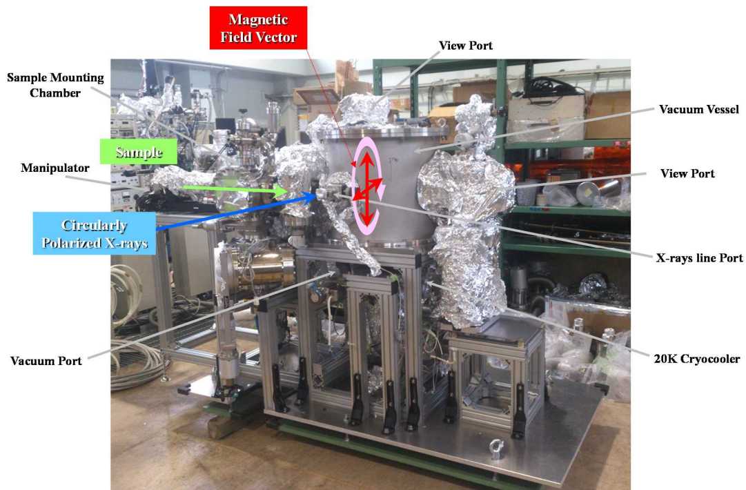
Fig. 3.21 Photograph of the newly developed system. Circularly polarized X-rays are delivered in the direction of the arrow.
