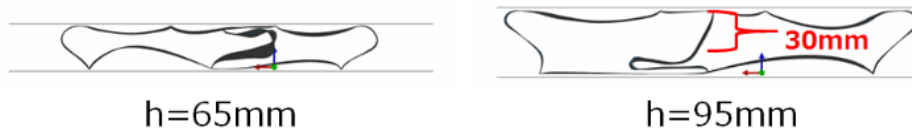
Fig. 5-3-6 Relationship between height and buckling length
