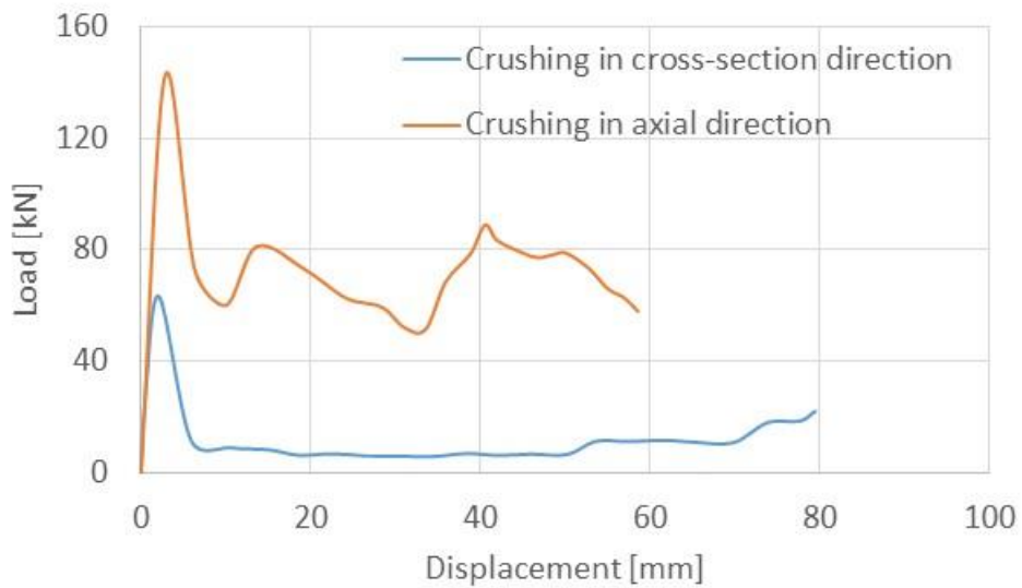
Fig. 3-2-2 Influence of difference in crush form on impact absorption behavior
