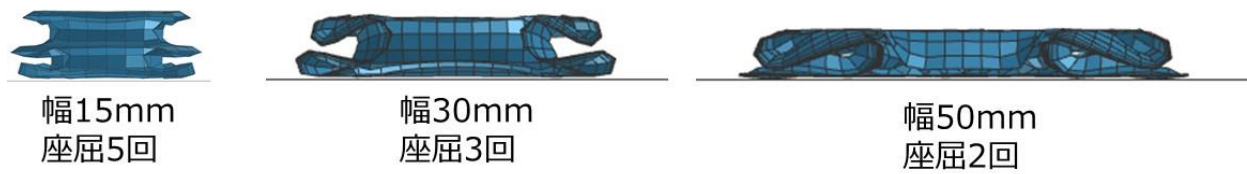
Fig. 4-4-5 Comparison of buckling mode (width)
