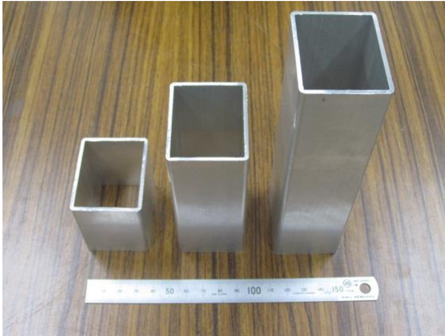
Fig. 3-2-3 Shape of specimen of shaft crush impact absorbing member
